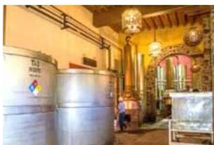
After fermenting the juice in large tanks, Tequila is distilled in archaic copper stills in small batches. As in all distillery processes the preliminary and follow-up distillate is discarded and only the central part used. Good tequila is distilled twice, which means the distillate obtained is then processed once again.
