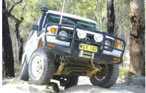
Picture 14: Rigid axle with leaf springs, articulated
