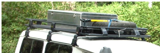
Picture 45: ARB roof rack with 6 supports
