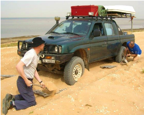
Picture 75: Recovery with 4 recovery boards
