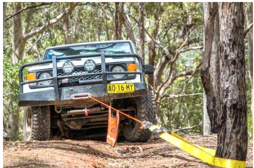
Picture 27: Winch recovery with tree protector Source: https://www.supercheapauto.co.nz/p/ridge-ryder-ridge-ryder-tree-trunk-protector-5m-10000kg/347356.html
