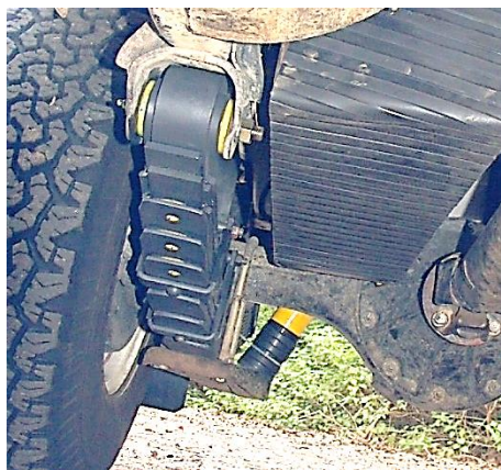
Picture 48: Protector for the shock absorber at the rear axle
