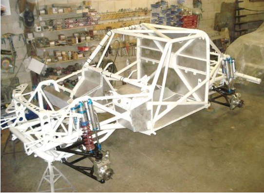
Picture 15 Independent suspension with „double wish bones“ front and rear
