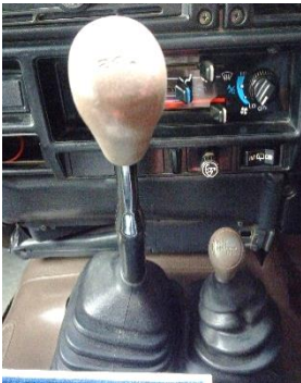
Picture 10: Lever for 4x4 and low-range (right)
