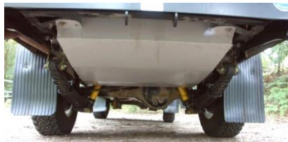
Picture 44: 180 l replacement tank
