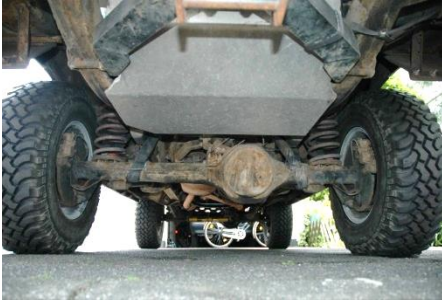
Picture 14: Rigid axle with coil springs
