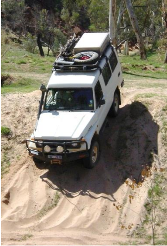
Picture 59: Steep descent in a vertical line
