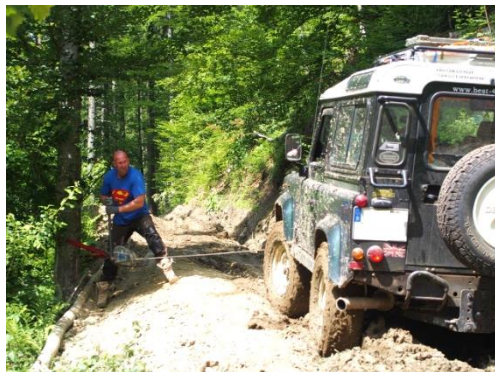
Picture 26: Recovery with cable pull
