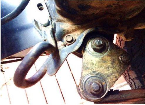
Picture80: Original recovery point of a Land Cruiser
