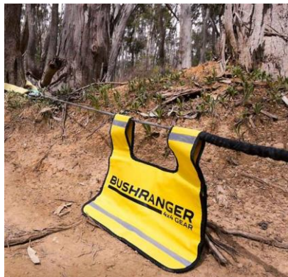
Picture 33: Rope damper at work
