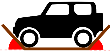
Picture 6 Approach and departure angle
