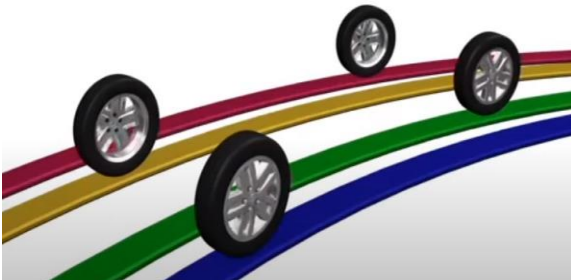
Picture 11: Different path for each wheel; Source Toyota University (You Tube)
