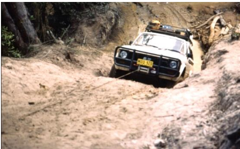
Picture 77: Self recovery with the winch
