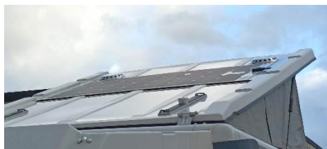
Figure 40 Flexible solar panel, installed with ventilation ( underway.ch )
