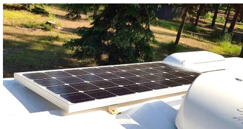
Figure 41 Rigid mono-crystalline panel (source: https://ousuca.com/camping-solaranlage-kaufen/ )
